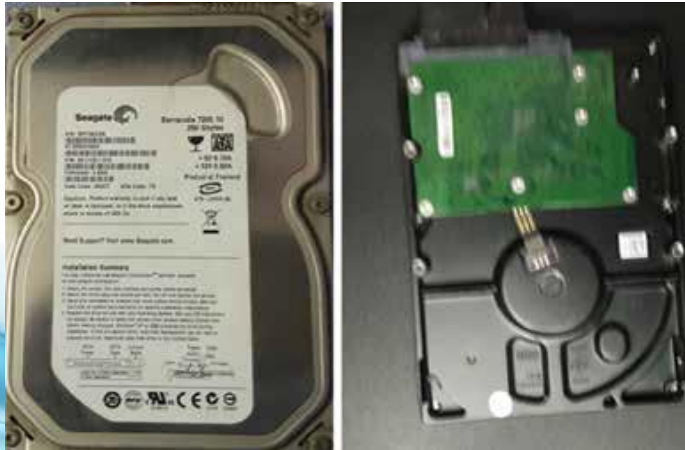
Two sided view of a sealed hard disk unit
